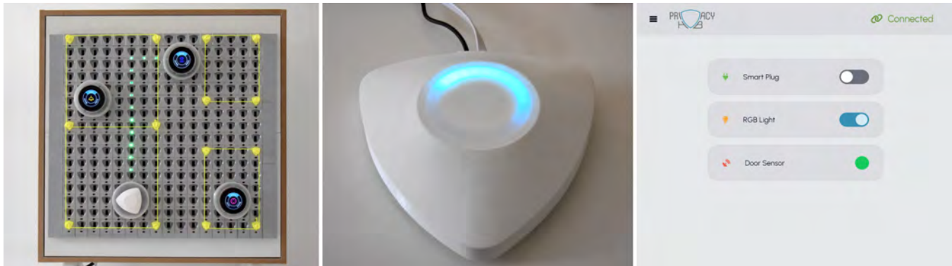
Figure 1: Left is the physical dashboard with yellow strings visualizing the floor plan and proxies representing the smart devices. Users can adjust privacy states by turning the proxy's ring; LEDs then indicate data streams. The top-right is the privacy hub, the system's communication unit, and the bottom-right is the web application for digital control.
