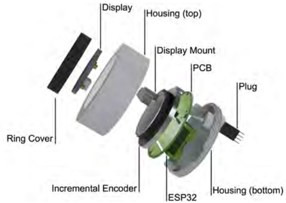
Figure 6: An exploded view of a proxy with its key components: The ring cover, incremental encoder, display, PCB, ESP32 microcontroller, and plug, all enclosed within the top and bottom housing.
